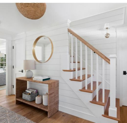
Our clients decided on a pre-engineered, prefinished floor system. It has a wood surface that can be sanded and refinished once or twice over a backing of plywood. It's a practical, more stable way to install wide boards in moist environments.
